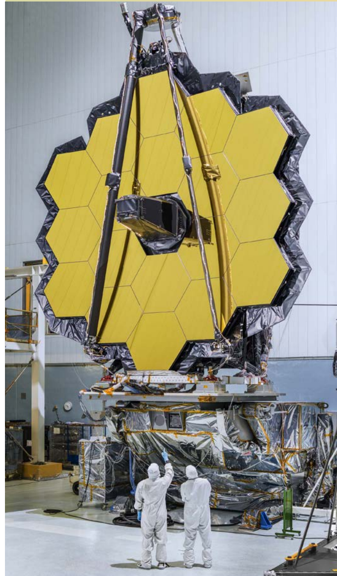
The primary mirror of NASA's James Webb Space Telescope, consisting of 18 hexagonal mirrors, looks like a giant puzzle piece standing in the massive clean room of NASA's Goddard Space Flight Center in Greenbelt, Maryland. (NASA/Goddard/Chris Gunn)
