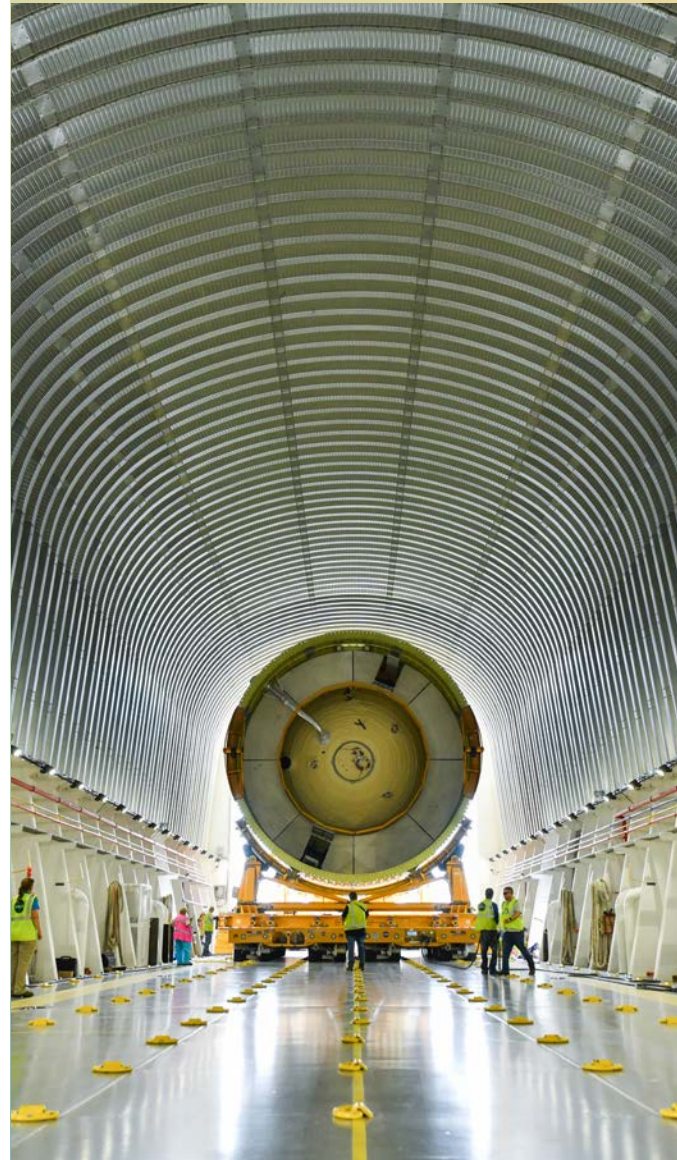
The liquid oxygen tank structural test article for the Space Launch System is loaded onto NASA's Pegasus barge (NASA/Jude Guidry)
