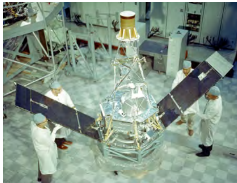
Mariner 2 under construction.
