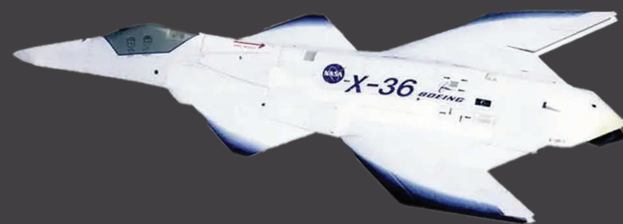
X-36 Tailless Fighter Agility Research Aircraft
