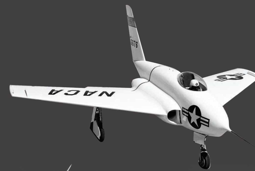
X-4 Bantam Semi-Tailless Aircraft
