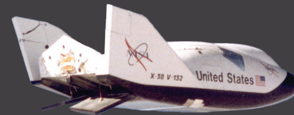
X-38 Prototype Crew Return Vehicle
